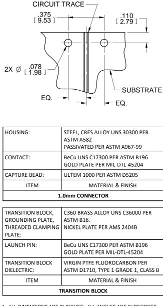
1. ALL DIMENSIONS ARE IN INCHES. ALL ANGLES ARE IN DEGREES. DIMENSIONS SHOWN IN BRACKETS [XXX] ARE IN MILLIMETERS.
